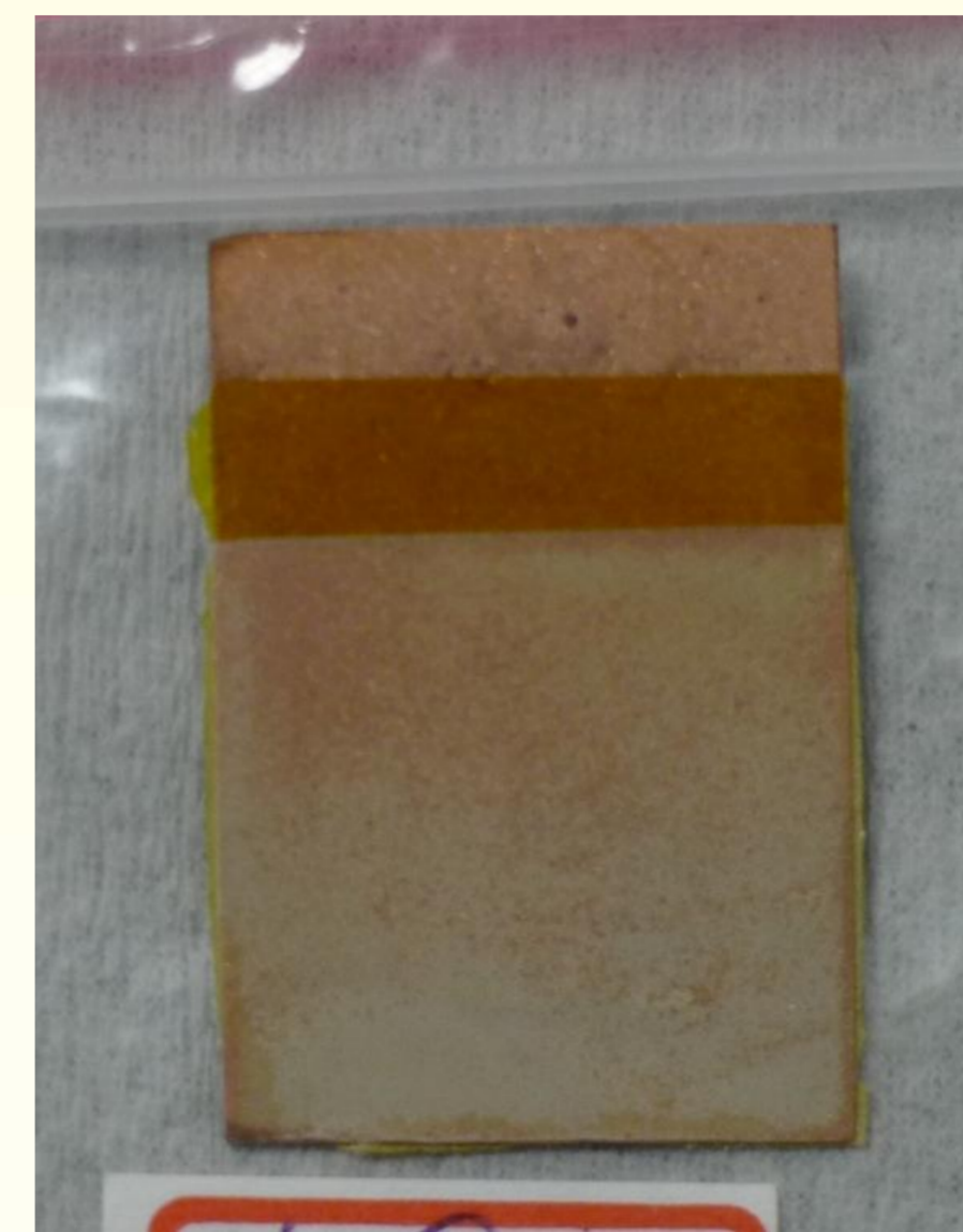
Figure 1. Picture of the hydroxide precursor with best deposition condition
