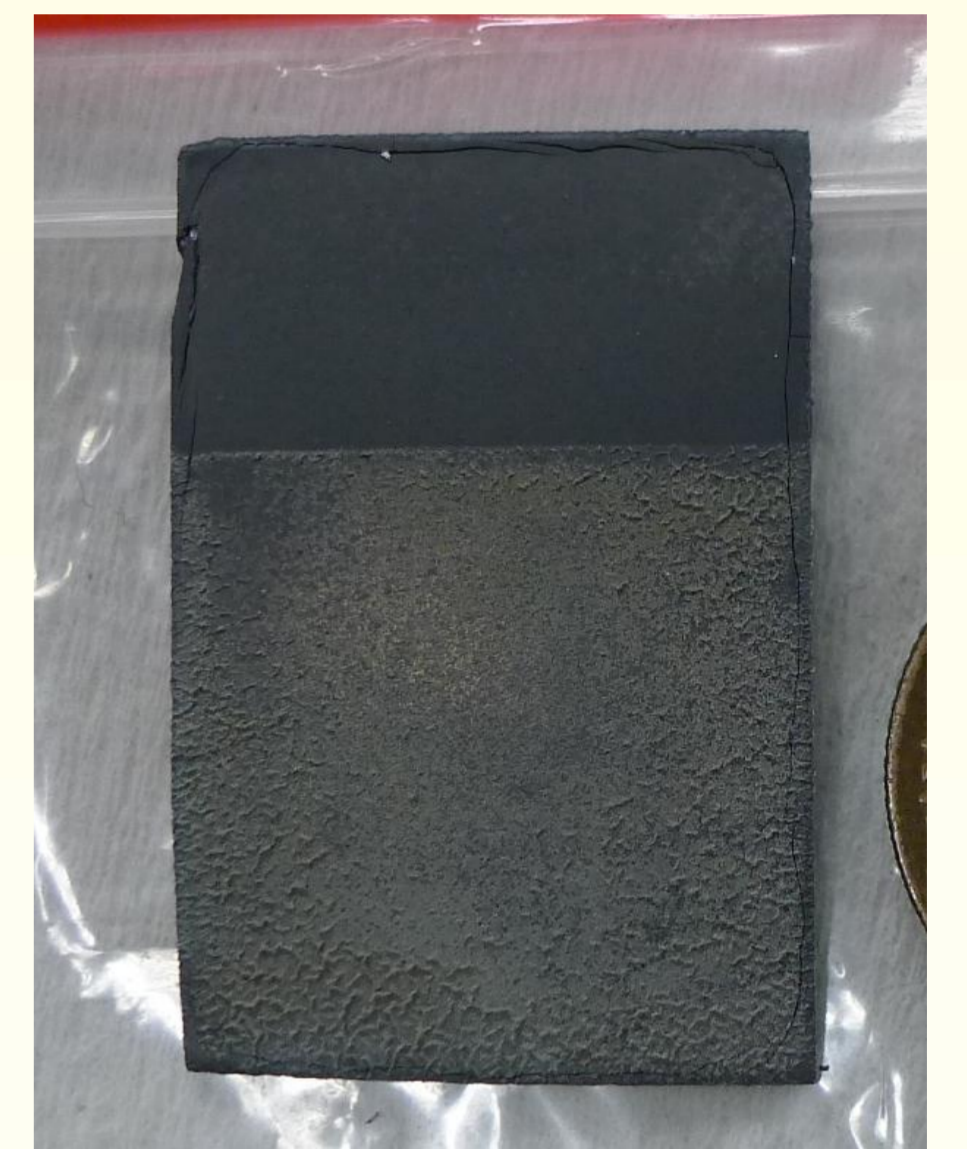
Figure 2. Picture of the thin film of perovskite oxide with best deposition condition after heat treatment at 900 °C
